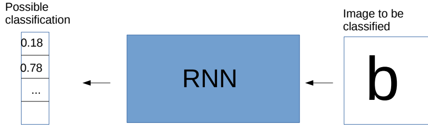
Figure 1: Depiction of the generative model and the Inverse Classification. For the Inverse Classification the generative network (in this case an RNN) reconstructs the character by using the temporal gradient information until it converges to a vector. A possible classification vector is represented in the left
